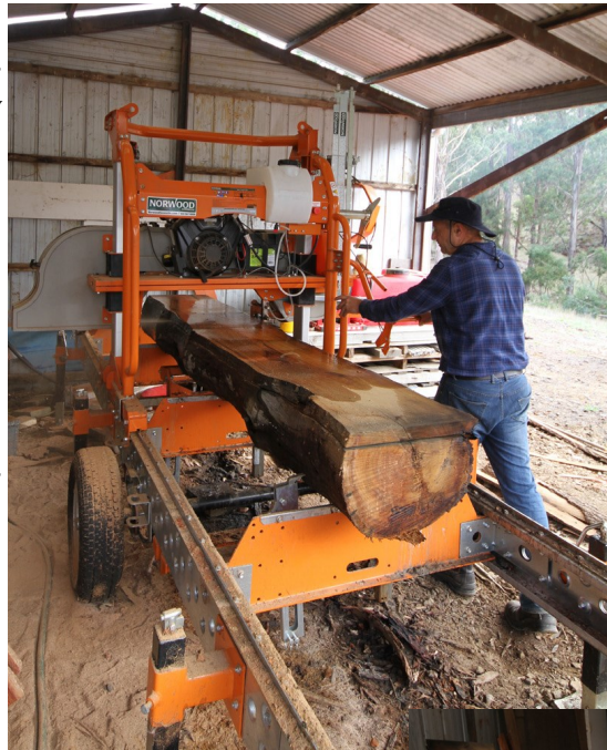
Rohan demonstrating the unique log manipulation capabilities of his Norwood Sawmill, and the resulting product as seen on the right.
