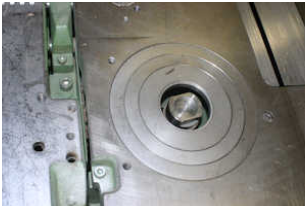
[Fig. 19. Router axle on a Robland combination machine. Its axle is 38 mm diameter and has two RPM settings, 3000 and 6000!]
