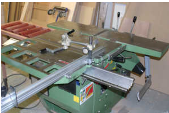
[Fig. 20. Overview of a Robland combination machine: Circular saw, router, planer, thicknesser and mortise cutter.]
