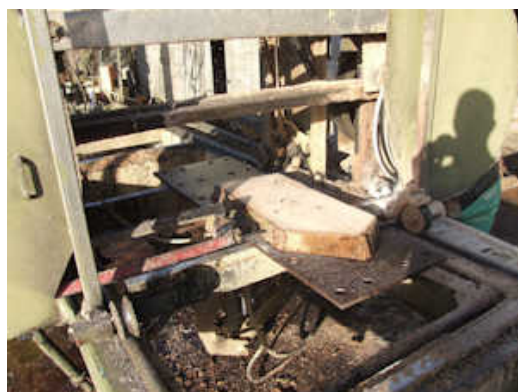
[Figs. 6,7. Sawing a short section using Erik Both's special aid. First, a cut through the heart is made, then boards are produced.]
