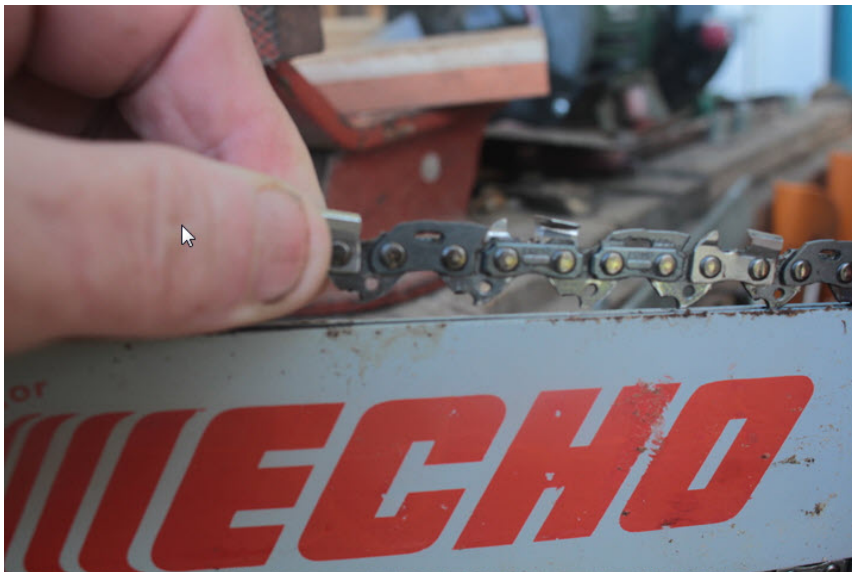
Fig.17. Play on the chain that's really pulled up hard.
