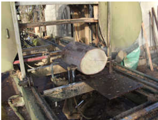
[Figs. 6,7. Sawing a short section using Erik Both's special aid. First, a cut through the heart is made, then boards are produced.]
