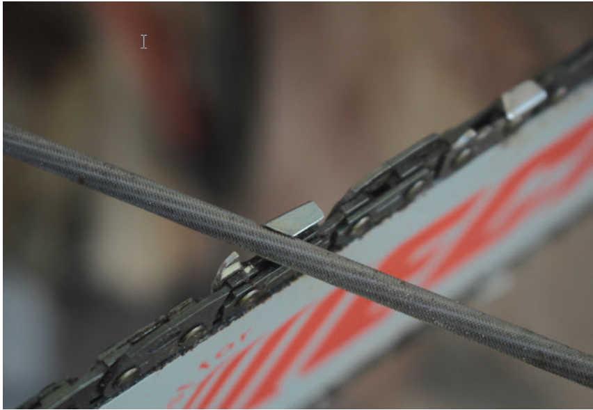
Fig.16. Way of sharpening teeth on the chainsaw
