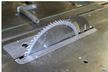
[Fig. 11. Circular saw on a Robland combination machine that weighs 400 kilos ~900 lbs): stable and as safe as a circular saw can be. On the right is the riving knife that will keep open the cut you just sawed. Able to saw cuts 80mm ~3 1/4" high.]
