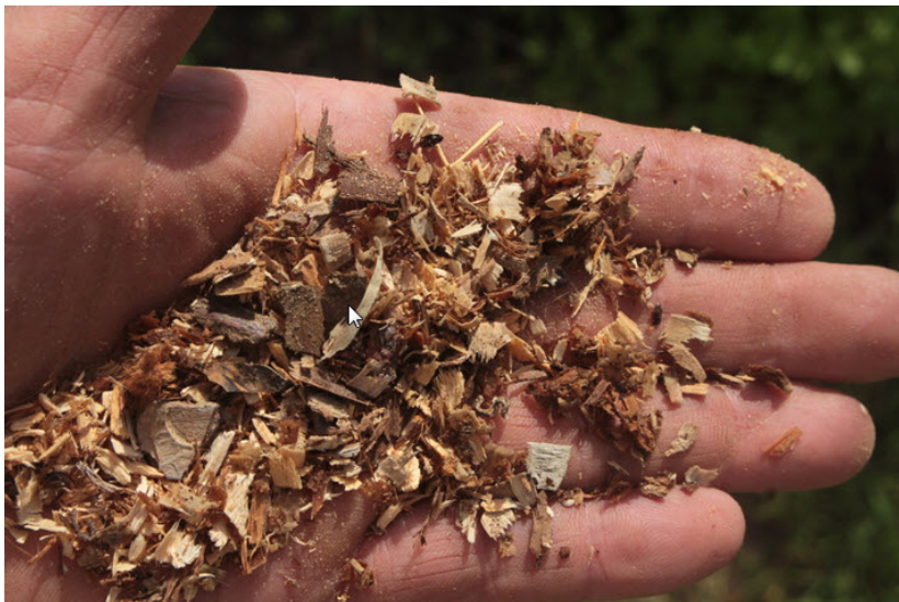
Fig.15. Crude shavings are proof that your chain teeth are well sharpened.
