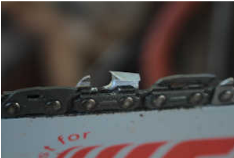
Fig.14. Showing a well sharpened tooth on a chainsaw.
