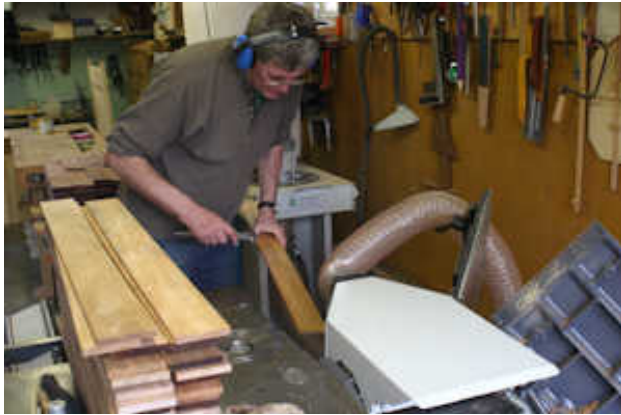
[Fig. 18. Working with a thicknesser. Note proper dust extraction and ear protection. Checking the dimensions never hurts!]
