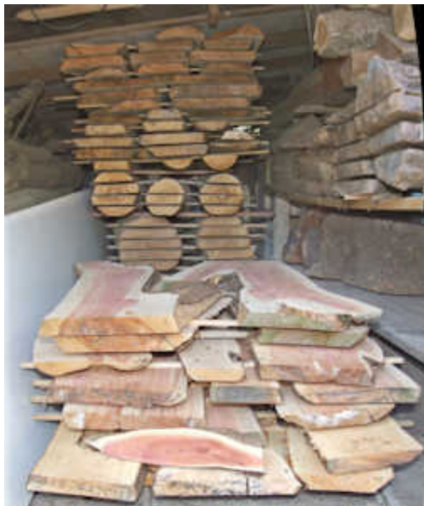
[Fig. 12. Wood drying in a shed. The boards are separated by narrow stiles to allow circulation of air, and prevent mould. We entertained some concern about the stability of the stack in the back.]
