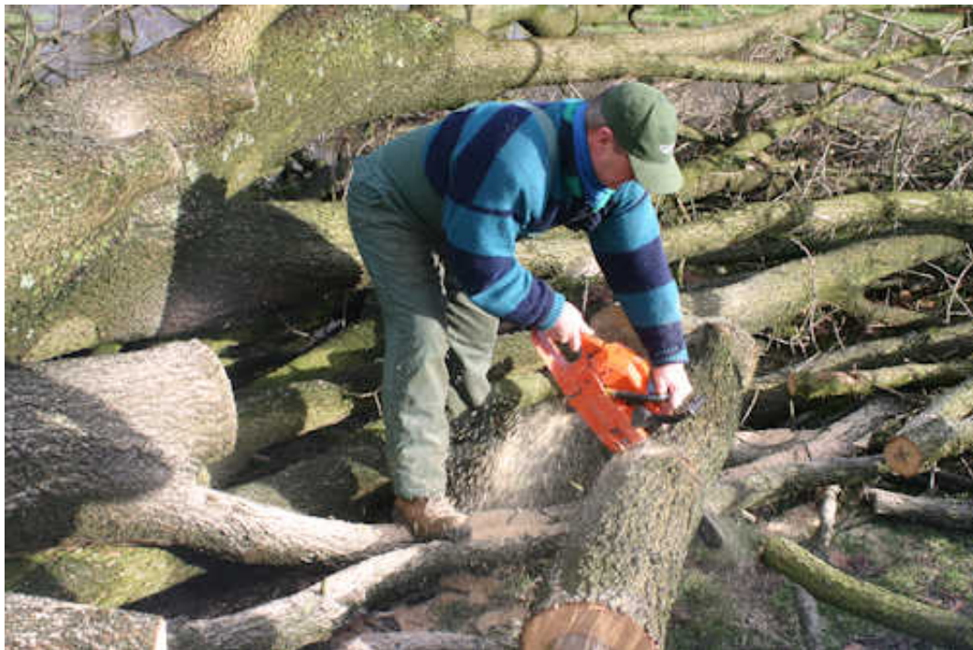
[Fig. 1. Use of protection gear. Harry Wissink is wearing a safety suit and safety boots and has supported the part he is bucking. The rough chips indicate his chainsaw is sharpened well.
