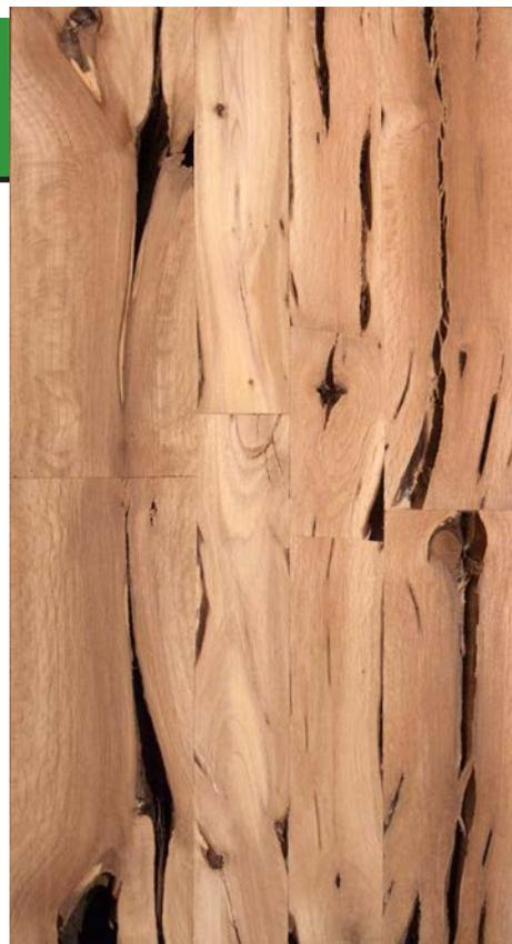
Longitudinal surface of a glued up *Lavandula angustifolia* wood specimen, containing both flat sawn and quarter sawn wood
