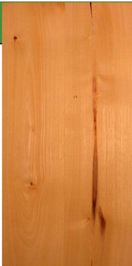
Longitudinal flat sawn and quartersawn surface of a glued-up *Choisya ternata* wood specimen
